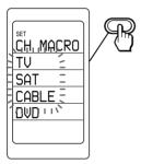
The selected component name appears. The macro labels flash. (To change the labels, press the SCROLL button repeatedly.)
